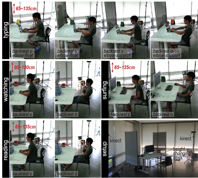
Figure 6: This figure illustrates 10 conditions used for pose capturing. We captured four actions (typing, watching, surfing, and reading) concerning sitting preference (using a backrest or not), lower arm positions (elbow supported or not), and height variations (desk height/monitor height). The poses were 3D captured with two Kinect devices.
