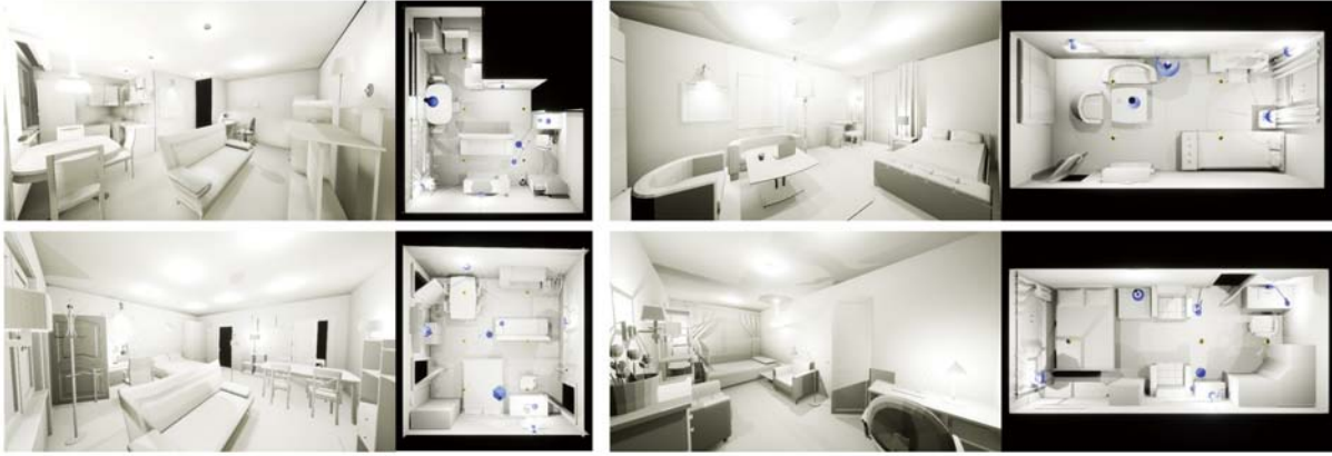
Figure 11: Diverse indoor scenes including lighting layout generated by our system. The four scenes are seen as a perspective view on the left and a top view on the right. In the top view image, local light is marked in blue and general light (ceiling light) is marked in yellow. The left column shows the living room and the studio, and the right column shows the two different private rooms.
