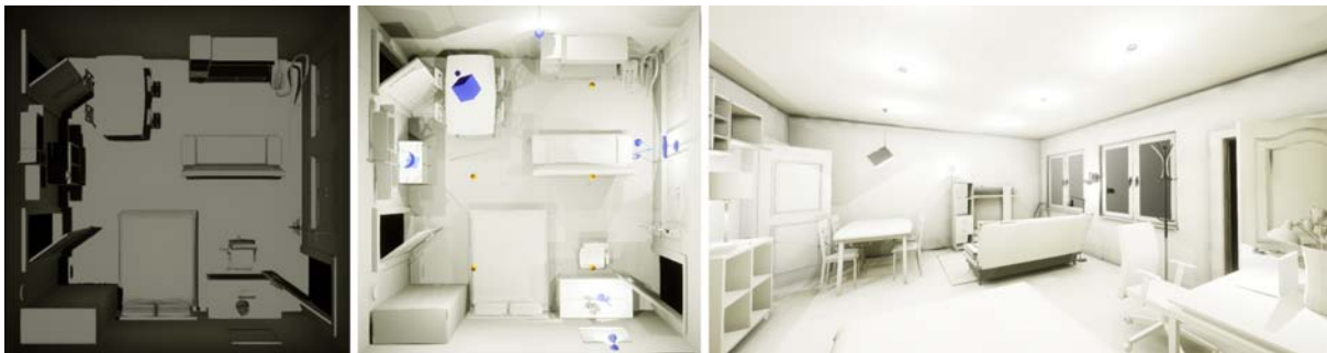
Figure 1: Left: Initial indoor scene with furniture installed (top view). Middle and right: Rendered scenes with lighting, for which the arrangement and intensity are automatically computed by our method. Lights are blue and yellow in the middle figure.
