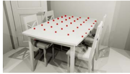
Figure 10: Sample points scattered at regular intervals to measure illuminance on the task plane.
